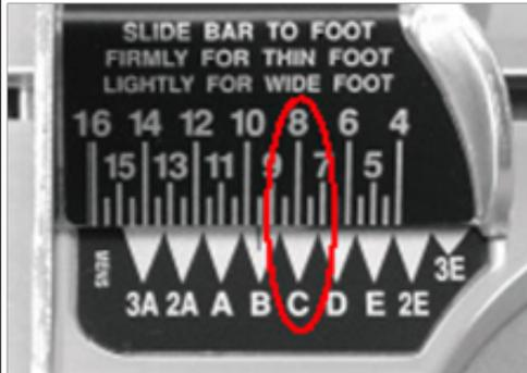
Slide the width bar firmly to the edge of the foot. Locate the shoe size (as determined in step four) on the movable width bar and view the width measurement indicated by the properly determined shoe size. If the shoe size falls between widths, choose a wider width for a thick foot, a narrower width for a thin foot.
