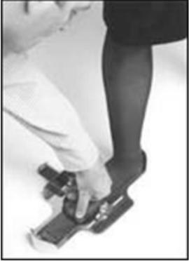
Press the toes flat against the base of the device and look straight down over the longest toe (not necessarily the first toe) to read toe length. Make sure the customer's socks are snug against the toes (without drawing the toes back) to yield an accurate measurement.
